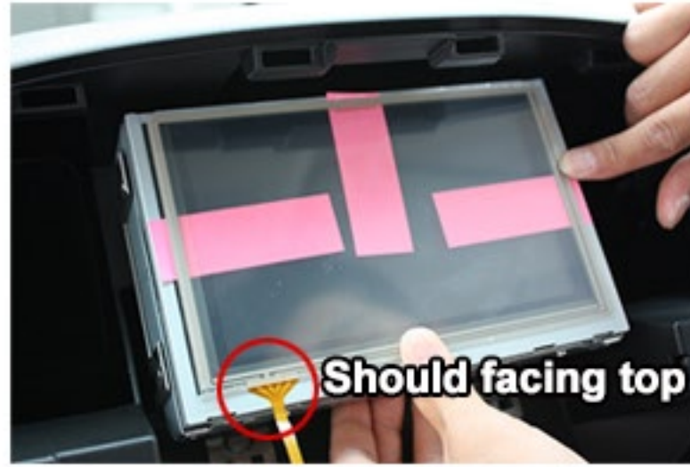
Once the panel has modified to the screen size put it over the screen. Make sure Touch Film faces top.
