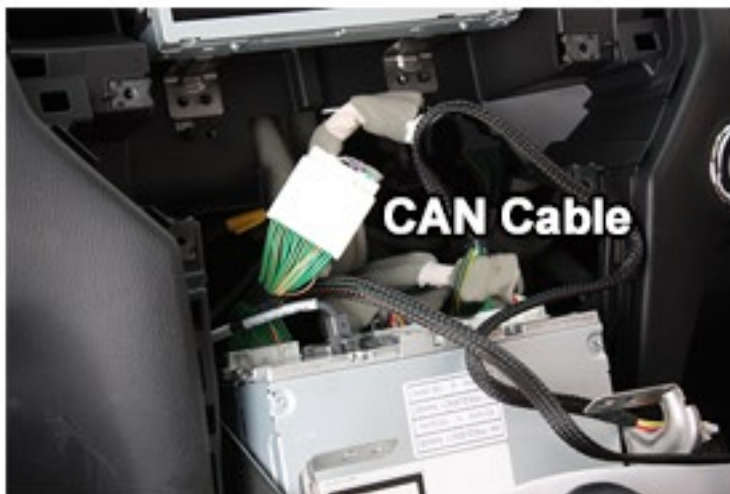
From bypass cable, conect Can port (2Pin) to the Interface box.
