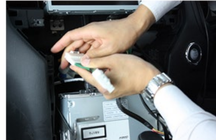
Conect provided bypas CAN cable to audio deck's Main cable
