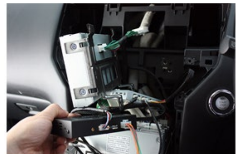
Connect provided RGB cable between Interface & NAV boxes
