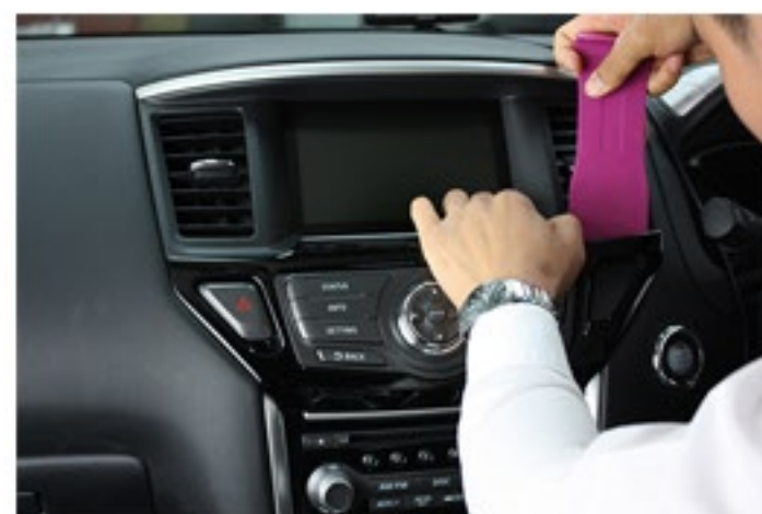
Remove control panel trim
