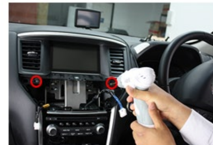
Remove bolts those holding Air Con trim
