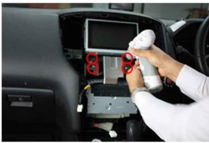
Remove 4 bolts those holding audio & monitor (the bracket)
