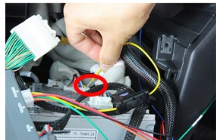
From NAV power cable (6pin). connect Nav Yellow to marked wire *Use test light to confirm the power.
