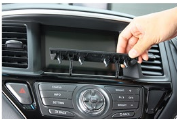
Pull out the trim in front of the screen
