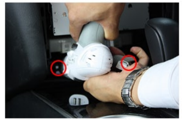
Under the audio, remove those bolts that holding audio deck.
