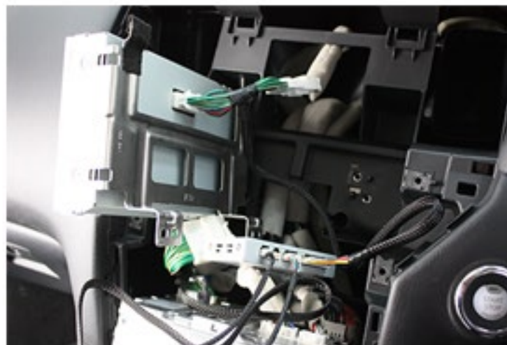
Do the same with 24Pin RGB cable to back of the monitor . Both 24 Pin & 32 Pin cable will be connected as Bypass between audio deck & Monitor
