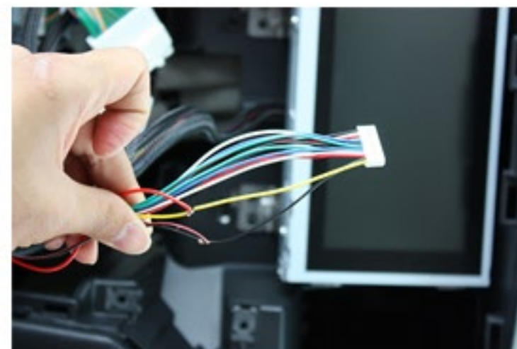
From NAV Power cable (6pin), connect NAV Red to RGB (from 24pin main cable) Yellow and NAV Black to RGB Black
