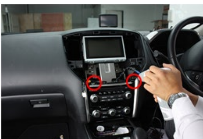
Remove those 2 bolts, that holding bottom panel trim
