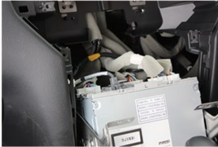
Pull out Audio deck and disconnect Main / CAN cable & RGB Cable
